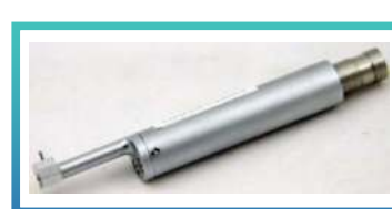
SRG4600-300 Small Hole Stylus. For use in small holes under 2mm diameter and max depth of 9mm.
