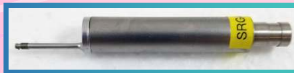
SRG4600-300 Small Hole Stylus For use on small holes under 2mm diameter and max depth of 4mm
