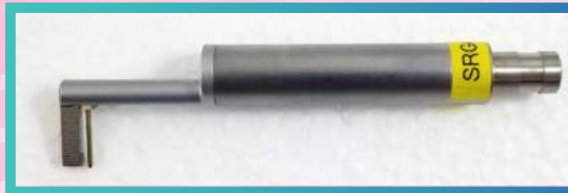
SRG4600-200 Deep Groove Stylus For use on deep grooves with min. width of 3mm and max depth of 10mm. Must use with support stand
