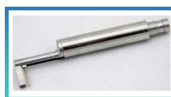
SRG4600-200 Deep Groove Stylus. For use on deep grooves with min. width of 3mm and max depth of 10mm. Must be used with support stand shown below
